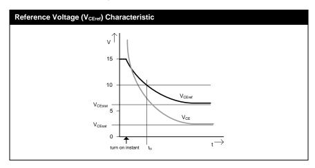
After  $t_{bl}$  has passed, the  $V_{CE}$  monitoring will be triggered as soon as  $V_{CE} > V_{CEref}$  and will turn off the IGBT. The error memory will be set, and the output PRIM\_HOLD\_OUT changes to the HIGH state. Possible failure modes are shows in the following pictures.
