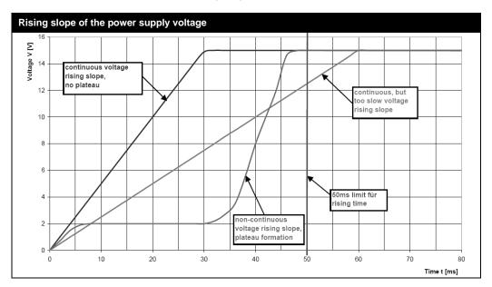
If the power supply is able to provide a higher current, a peak current will flow in the first instant to charge up the input capacitances on the driver. Its peak current value will be limited by the power supply and the effective impedances (e.g. distribution lines), only.
